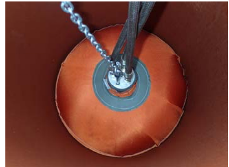
Figure 4 – Pressurise Dual Gas Bag during FAT
