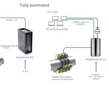
Swarm® S1's unique design allows for installation on critical areas such as top of welds, heated weld zones, elbows and T-pieces to monitor and detect:
