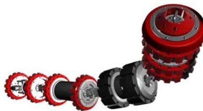
Figure 3 – Example of a High Resolution MFL tools
