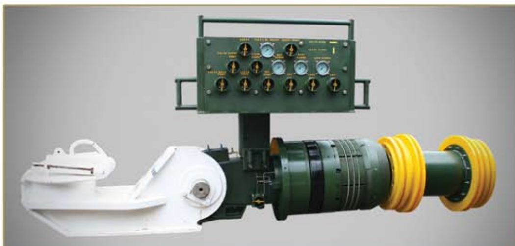
36" ROV Deployed PRT - Shown With De-watering Pig Attached & Detachable ROV Operated Control Panel
